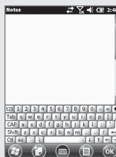
This input method displays an on-screen keyboard that can be used to input characters by tapping the screen using the stylus pen.
