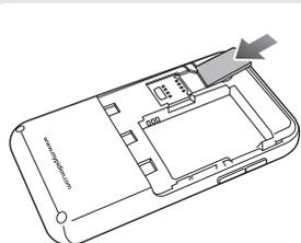
Insert the SIM card with its gold contacts face down. Its cut off corner should match the cut off corner in the slot.
