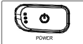
This button is used to turn the printer on and off.
