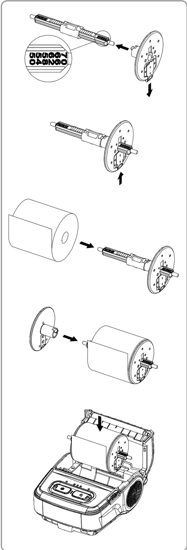
1) Release the disk lock and insert it into the spindle as shown in the picture.. (Position the disc so that the media width is equal to the scale on the spindle.)
