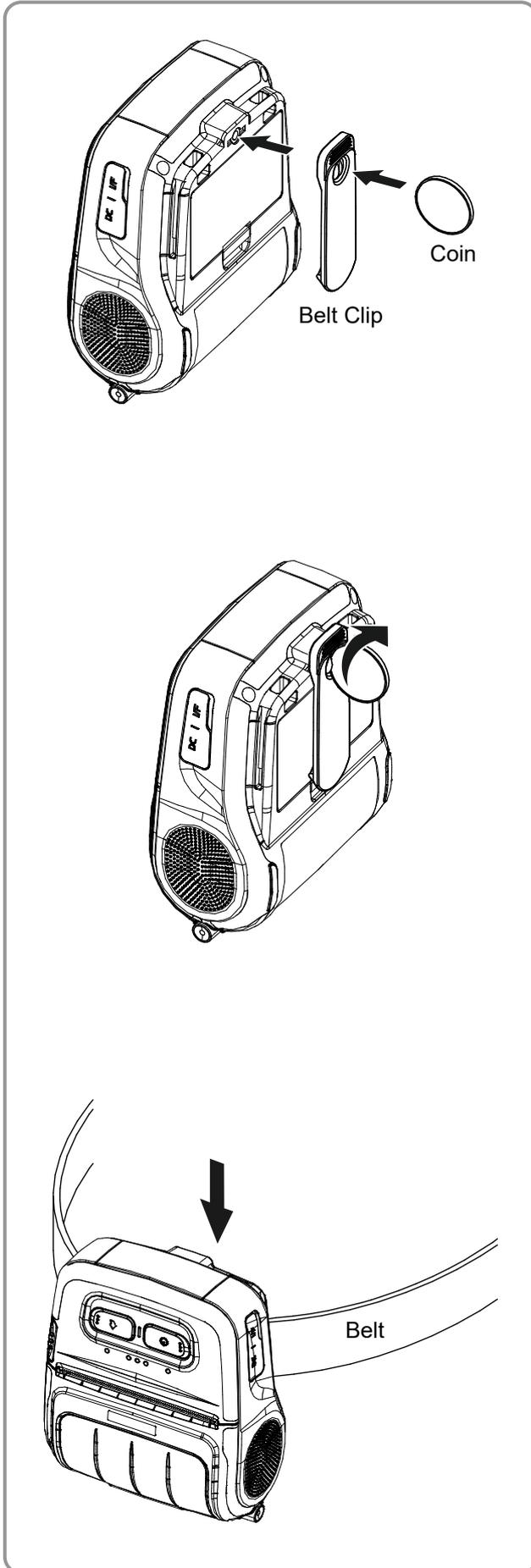
1) Insert the belt clip screw to the belt clip mounting hole.
