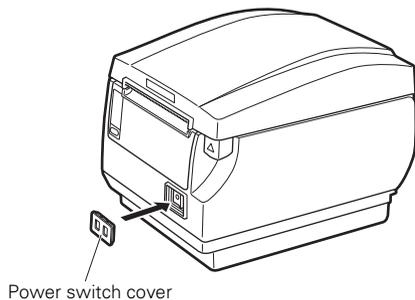
Put a screwdriver or other pointed object into the grooves on the power switch cover to remove it.
