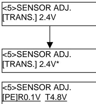
(3) Press and hold the **[RESTART]** or **[FEED]** key for about 3 seconds aligning a blank part of print area with the Feed Gap Sensor.
