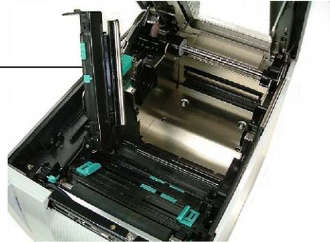
5. Remove the jammed media from the printer. **DO NOT USE** any sharp implements or tools as these could damage the printer.
