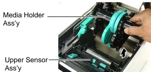
3. Raise the Release Lever and remove the Media Holder (Left).
