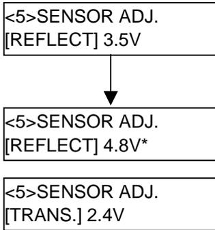
(3) Press and hold the **[RESTART]** or **[FEED]** key for about 3 seconds aligning a blank part of print area with the Black Mark Sensor.
