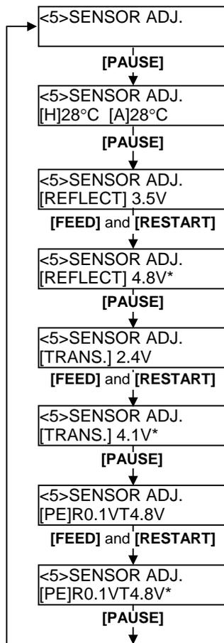
The Sensor Adjustment Mode contains sub menus for displaying the current status of each sensor and for storing “media level” voltage and “no media level” voltage. Each time the [PAUSE] key is pressed, the sub menus are displayed sequentially.
