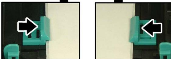
10. Lower the Upper Sensor Ass'y until the Upper Sensor Lever clicks into position.
