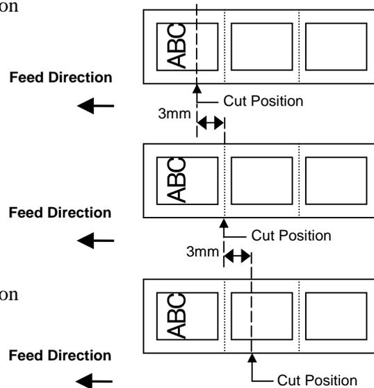
**• Example of Strip Position Fine Adjustment**When setting +3.0 mm
