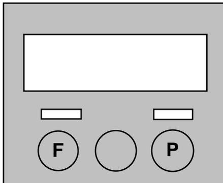
1. While holding down the **[FEED]** and **[PAUSE]** keys, turn on the printer.
