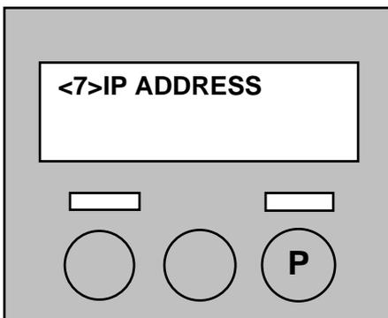
4. Press the **[PAUSE]** key to enter the IP Address Setting Mode.
