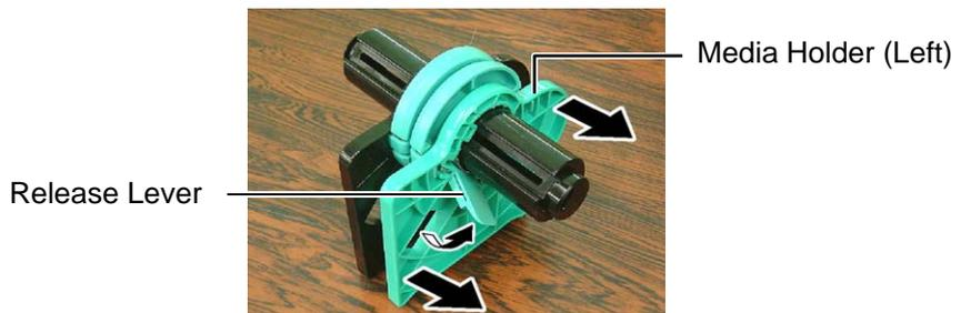
4. Insert the Media Shaft into the core of a media roll.
