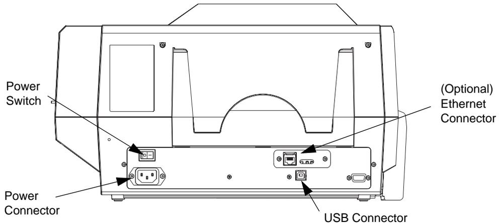
2. If your printer includes the optional Ethernet Adapter as well as the standard USB connection, use **either** the supplied USB cable or a standard Ethernet cable to connect the printer to a corresponding port on the computer or network.
