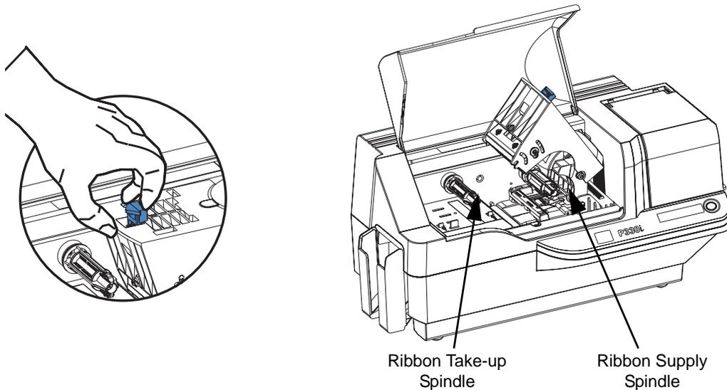
3. Locate the Ribbon Supply Spindle and the Ribbon Take-up Spindle (see above). Load ribbon onto the supply spindle (under the print head carriage) **flange side in**, and load the empty core (with tape attached) onto the take-up spindle. Make sure the ribbon comes off the top of the supply spindle and feeds to the top of the take-up spindle.
