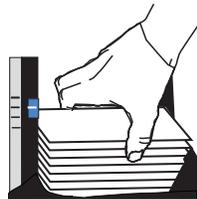
6. Note that there will be a “gap” in the card stack, with several cards lying flat and the cards above angled upward, as shown in the exaggerated drawing below. **This is normal** and ensures proper feeding.
