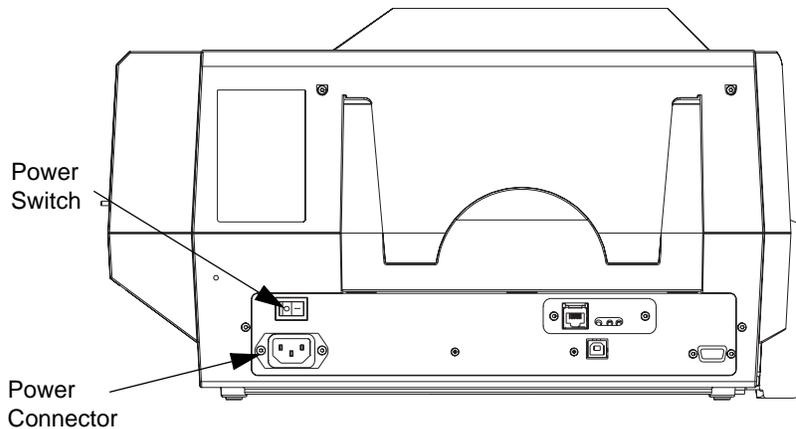
1. Place the Printer's power switch in the OFF ( **O** ) position.
