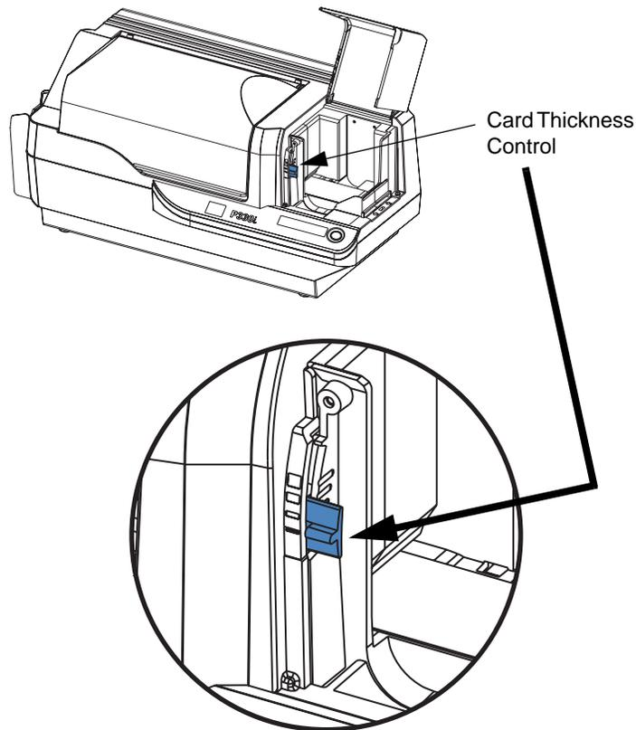
3. There are four detents to set the position of the Card Thickness Control. Slide the Card Thickness Control to the position corresponding to the following:
