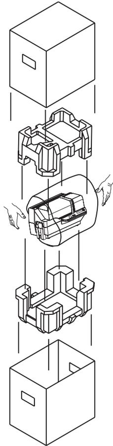
5. Lift the printer out of the carton by holding it with both hands.
