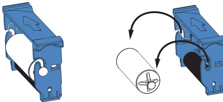
4. Install new cleaning roller into the Card Cleaning Cartridge. To avoid contamination, always hold the cleaning roller by the ends. (For replacement cleaning rollers, please refer to the Media List on the Windows Drivers and User Documentation CD supplied with this printer.)
