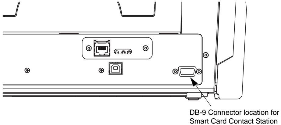
An attached external Smart Card Programmer can be used to program Smart Card chips. The following table shows the Smart Card Contact Points.
