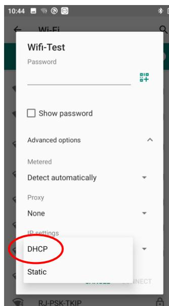
2. Select "Static" to customize the IP address. This will help to avoid the network failure caused by the duplication of the IP address in the LAN or the disable of the DHCP service in the router etc.
