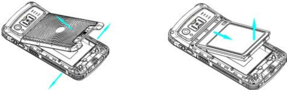
Step 1: Hold down the Power key for 5 seconds and then tap "Power off" to turn off the terminal. Slide the battery cover latch to the unlock position and remove the cover.
