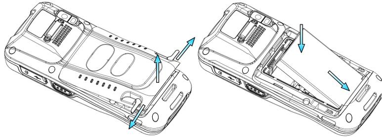
Step 1: Unlock the battery cover latches as shown in the figure above and then remove the cover.
