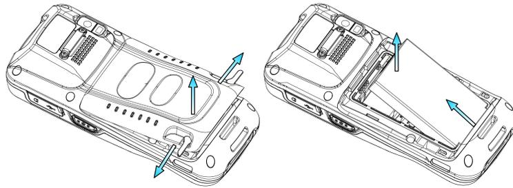
Step 1: Hold down the Power key for 5 seconds and then tap “Power off” to turn off the terminal. Unbuckle and loosen the hand strap. Unlock the battery cover latches and remove the cover.
