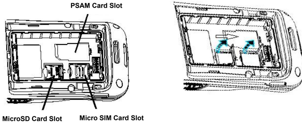
Step 1: Unbuckle and loosen the hand strap. Unlock the battery cover latch and remove the cover and battery. Slide the slot cover rightward and Lift the left end of it.
