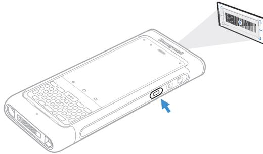
4. Release the Scan button when the computer beeps, and the Scan Status LED briefly turns on. The bar code information is entered into the application in use.
