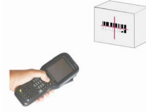
The Falcon X3 Imager uses an intelligent aiming system pattern, similar to those on cameras, indicating the field of view, which should be positioned over the code:
