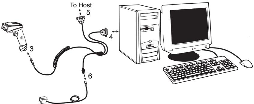
4. Plug the serial connector into the serial port on your computer. Tighten the two screws to secure the connector to the port.
