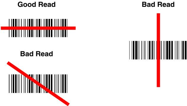
The best focus point for reading most code densities is about 5 inches (12.7 cm) from the unit. To read single or multiple symbols (on a page or on an object), hold the imager at an appropriate distance from the target, pull the trigger, and center the aiming line on the symbol.
