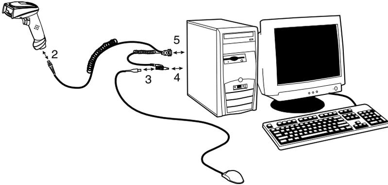
3. Unplug the mouse or keyboard from the computer. Plug the mouse or keyboard into the power tap on the scanner cable.
