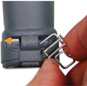
2. Gently turn the cable clip counter-clockwise and push the cable clip all the way through the strap hole.
