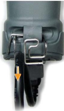
2. Unhook the left part of the cable clip from the strap hole then turn it clockwise. While in turning motion, push the cable clip all the way through.
